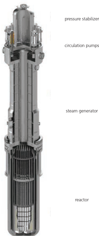
Fig. 41 Babcock & Wilcox mPower unit cross section (source: B&W promotional materials).
